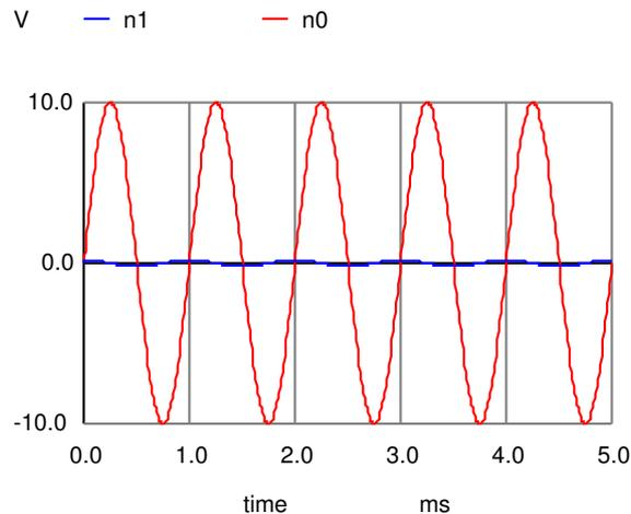
Figure 3: Input and output of the RC filter.
