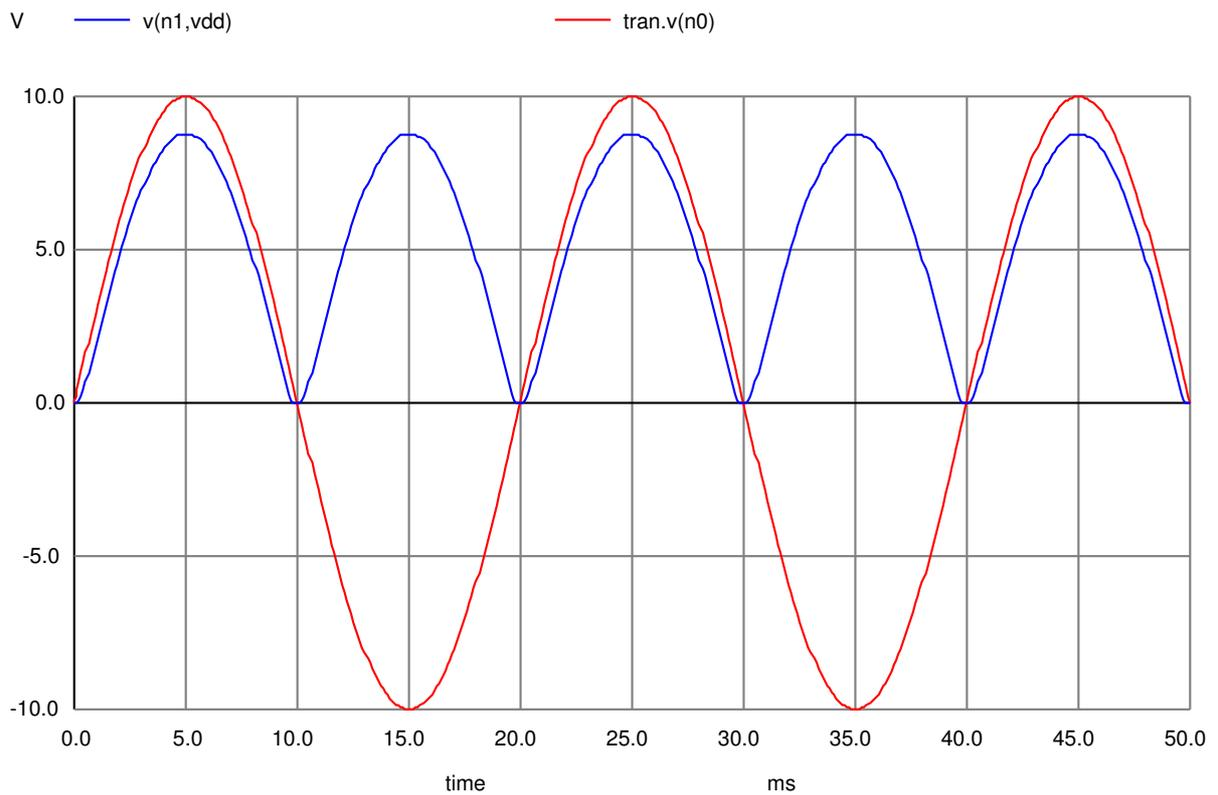
Figure 7: Source voltage transient and voltage across R1
