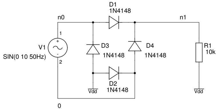
Figure 6: A full wave rectifier.
