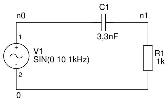
Figure 1: A simple RC filter.
