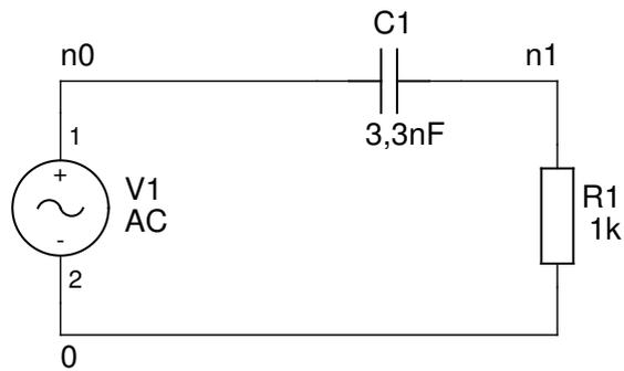
Figure 4: Filter for AC simulation.
