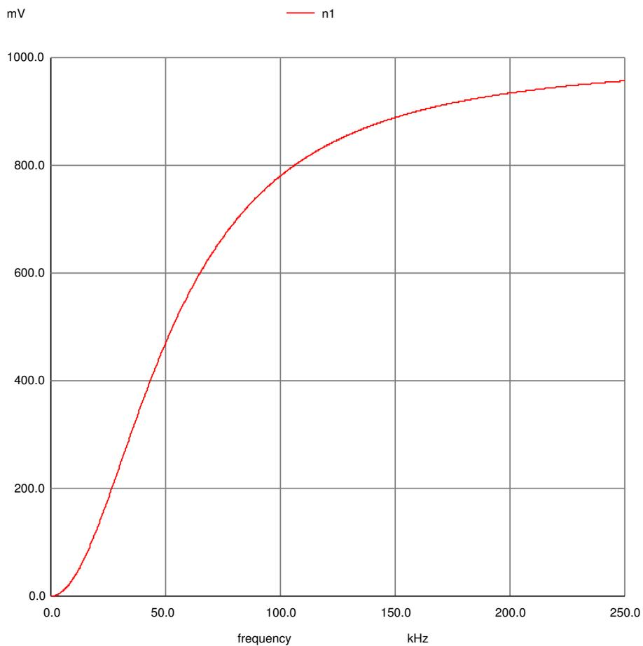
Figure 5: Frequency analysis of the RC filter.
