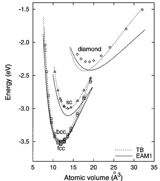
FIG. 7. Comparison of *ab initio* (LDA), TB, and EAM-calculated equations of state of the fcc ( $\square$ ), bcc ( $\circ$ ), sc ( $\triangle$ ), and diamond ( $\diamond$ ) structures of Cu around equilibrium.
