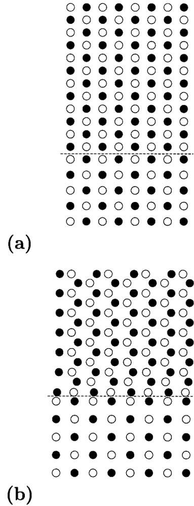
FIG. 15. Simulated structures of epitaxial Cu films on an fcc(001) substrate. The filled and open circles mark atomic positions in alternating (200) planes. The dashed line shows the interface between the substrate (below the line) and the film (above the line). The  $[010]_{\text{fcc}}$  direction is normal to the paper. (a)  $a/a_0 = 1.07$ ; the film has a deformed fcc structure. (b)  $a/a_0 = 1.24$ ; the film has an hcp structure.
