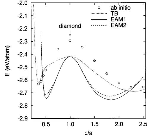
FIG. 12. Comparison of *ab initio* (LDA), TB, and EAM calculations of the energy of diamond Cu along the tetragonal deformation path. Calculations were performed at a constant volume corresponding to the equilibrium diamond structure.
