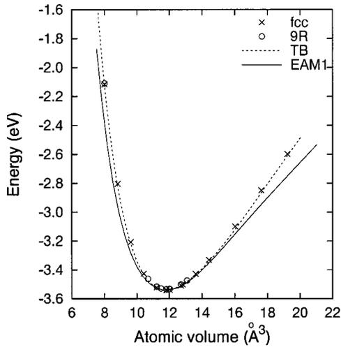
FIG. 8. Comparison of *ab initio* (LDA) ( $\times$ ,  $\circ$ ), TB, and EAM1-calculated equations of state of the fcc and 9R structures. In the range shown, the equations of state of both structures are practically identical.
