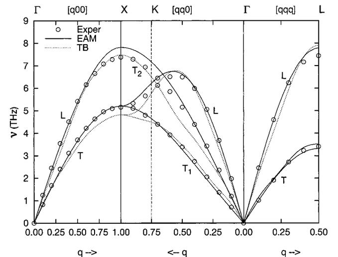
FIG. 2. Phonon dispersion curves calculated with the EAM1 potential and by the TB method. Experimental points ( $\circ$ ) measured by neutron diffraction at temperature 80 K are shown for comparison (Ref. 57).
