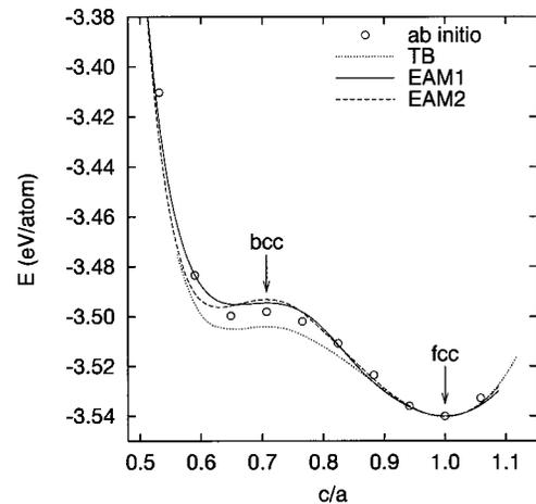
FIG. 10. Comparison of *ab initio* (LDA), TB, and EAM calculations of energy along the Bain path between fcc and bcc structures. Calculations were performed at a constant volume corresponding to the equilibrium fcc phase.
