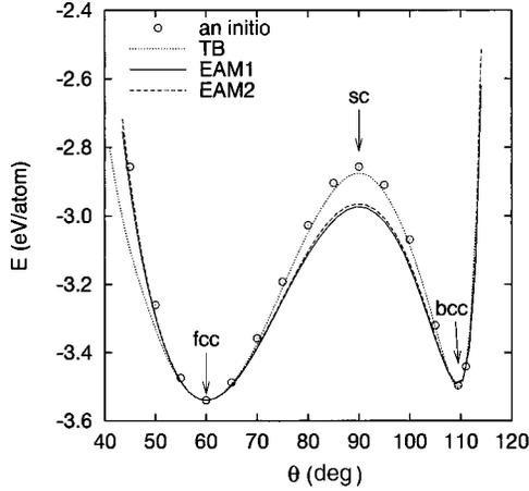
FIG. 11. Comparison of *ab initio* (LDA), TB, and EAM calculations of energy along the trigonal deformation path. Calculations were performed at a constant volume corresponding to the equilibrium fcc phase.
